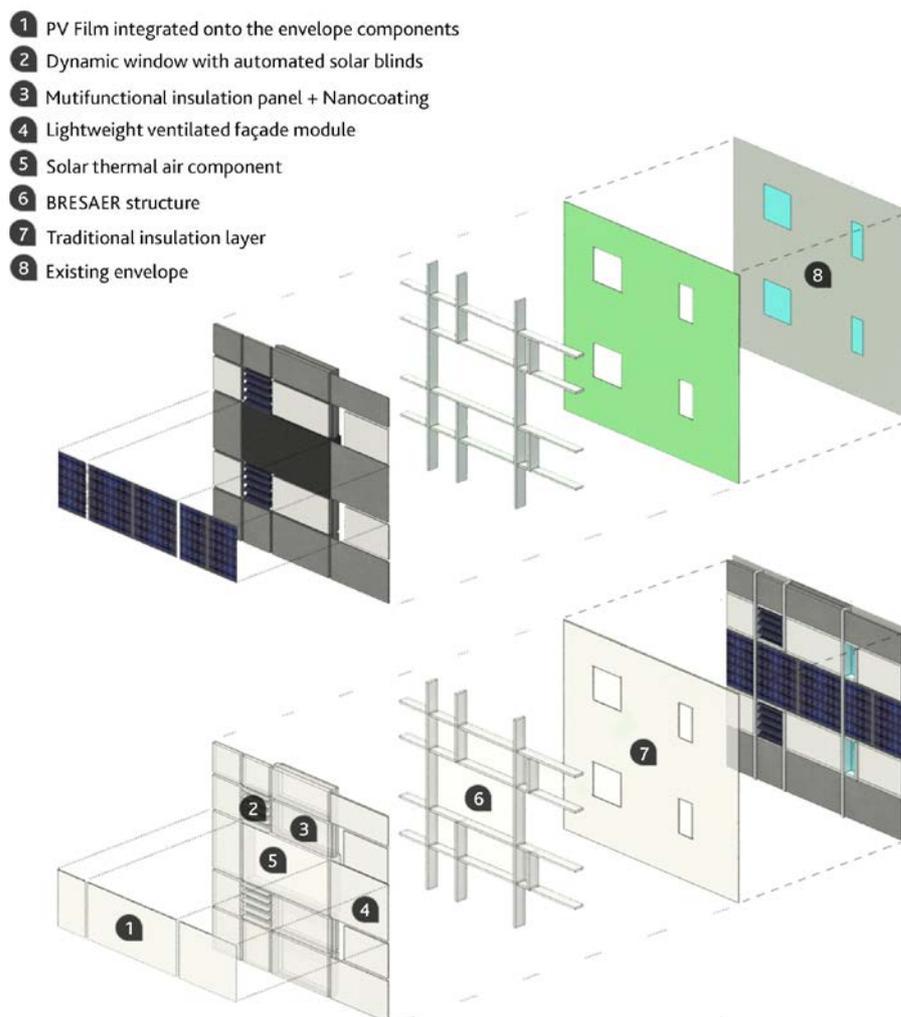
Figure 1. Schematic representation of the mostly active system. Image source: <http://www.bresaer.eu>
